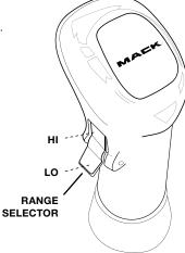
Failure to clutch or double-clutch when range shifting may result in damage to your vehicle's synchronizer.
